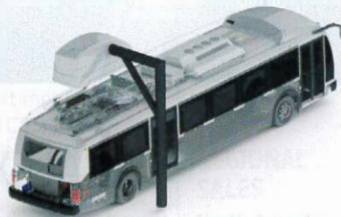
Fig. 2 - J3105-2 Infrastructure-Mounted Blade (Blade).
